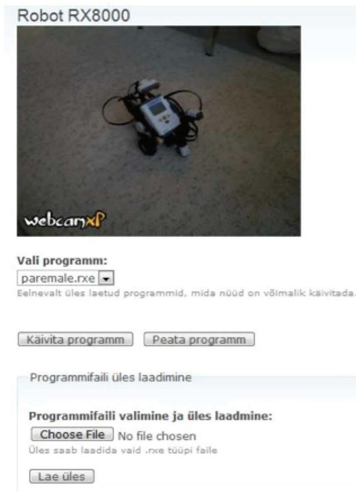
Fig.3. Prototype remote-control robot with video and control panel for students. Interface shows the possibility to choose a program from uploaded programs (Vali program). Below the choice box are buttons to start and stop the program (the latter is very useful button for beginners, as many newbie's programs tend to work in infinite loop). In the lower part of the screenshot is an interface for uploading a program.
