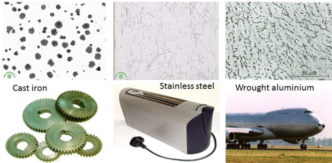
Fig. 3: Matching microstructure and component the very first day of materials science (microstructures [16,17], pictures [11,18])
